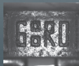
Coaxial spot lighting
