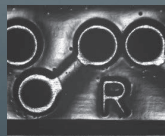
Coaxial spot lighting
