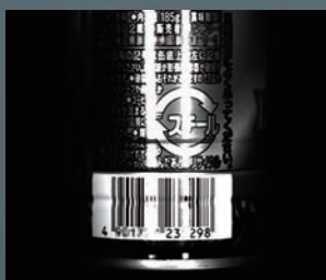
Bar light: Bar light x2 Oblique irradiation
