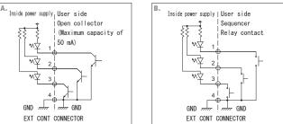
A current of about 10 mA is applied between connector pins 1, 2, and 3 and pin 4. Use an open-collector circuit with a capacity of about 50 mA to be on the safe side
