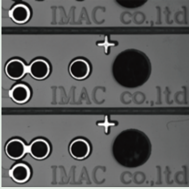
Narrow-angle light distribution type :IFVA-50W Shutter speed 1/10,000 Output:100%
