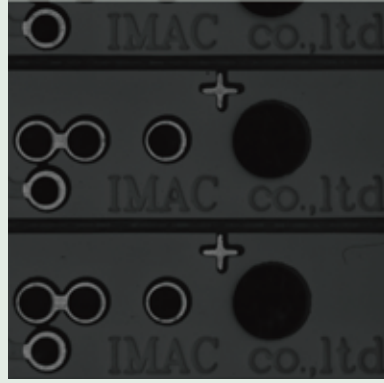
Diffuse light type:IFV-C50DW Shutter speed 1/10,000 Output:100%
