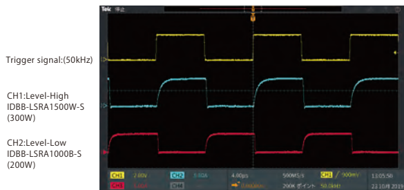
Even at 50kHz, each illumination responds quickly and without any delay.
