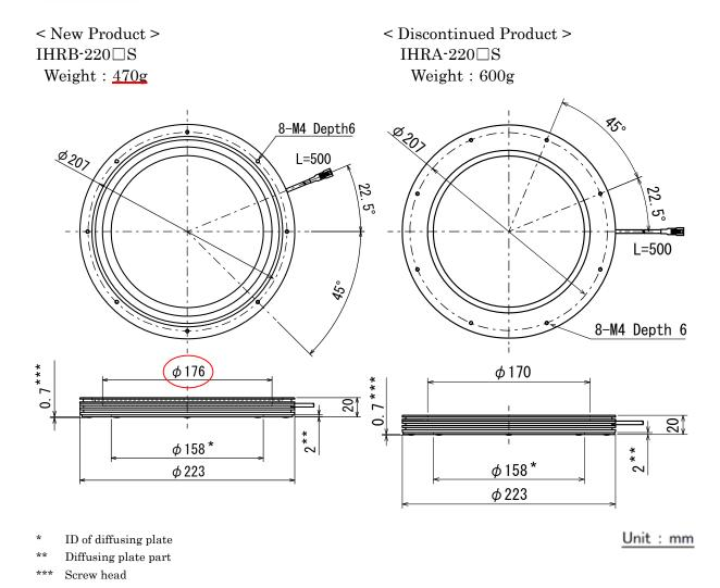
There are no other changes in optical characteristics, power consumption, brightness, or wavelength characteristics.
