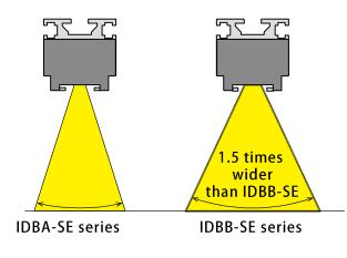
Compared to the discontinued model, the successor model has a 1.5 times wider light distribution angle, The light distribution angle will be approximately 1.5 times wider than that of the discontinued model.
